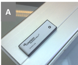
Picture 2A: Ideal tag placement with relatively large metal surface around the tag. 2B: Leave free metal area at least on the tag’s right side. 2C: Avoid placing the tag without metal area on its right side.
